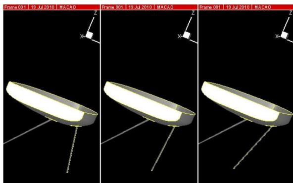
Figure 2 – CFD model with straight dagger-board
