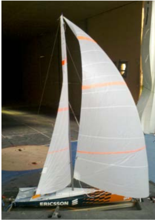
Figure 4: VO70 model scale yacht used for FEPV wind tunnel validation – comparison of calculated sail positions with physical measurements.
