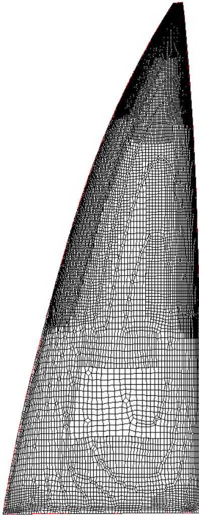
Figure 2 – Typical CFD surface mesh for a sail showing varying refinements along the height and additional refinements at the edges.
