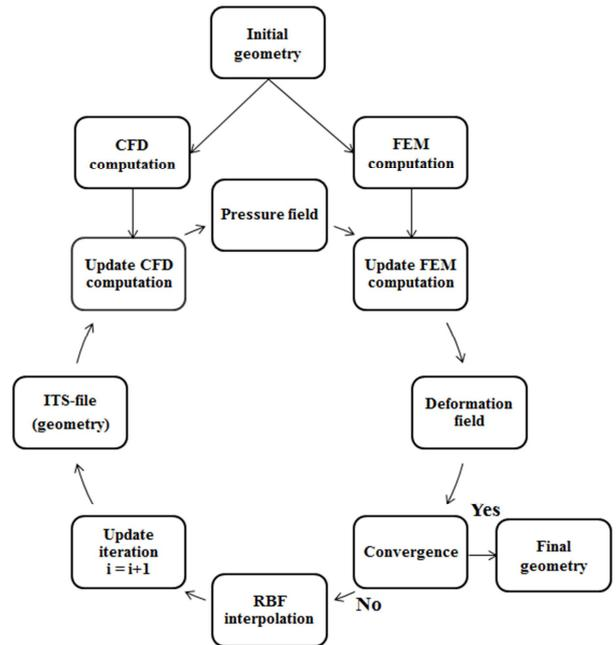
Figure 5 – Schematic representation of developed FSI method.
