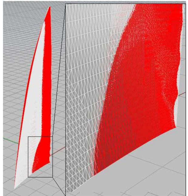
Figure 7 - Ripples at leading edge near tack of deformed shape of 3D.
