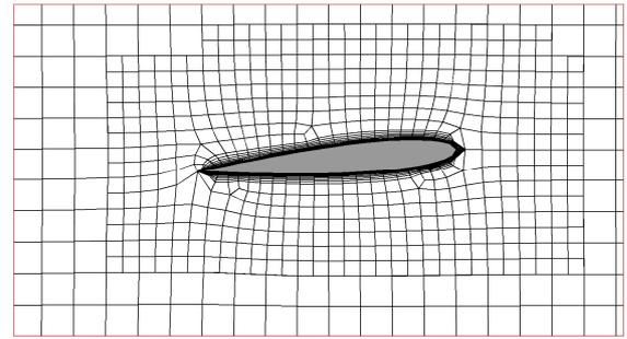
Figure 1 – characteristic mesh for NACA0012 profile, generated with HEXPRESS v2.11.
