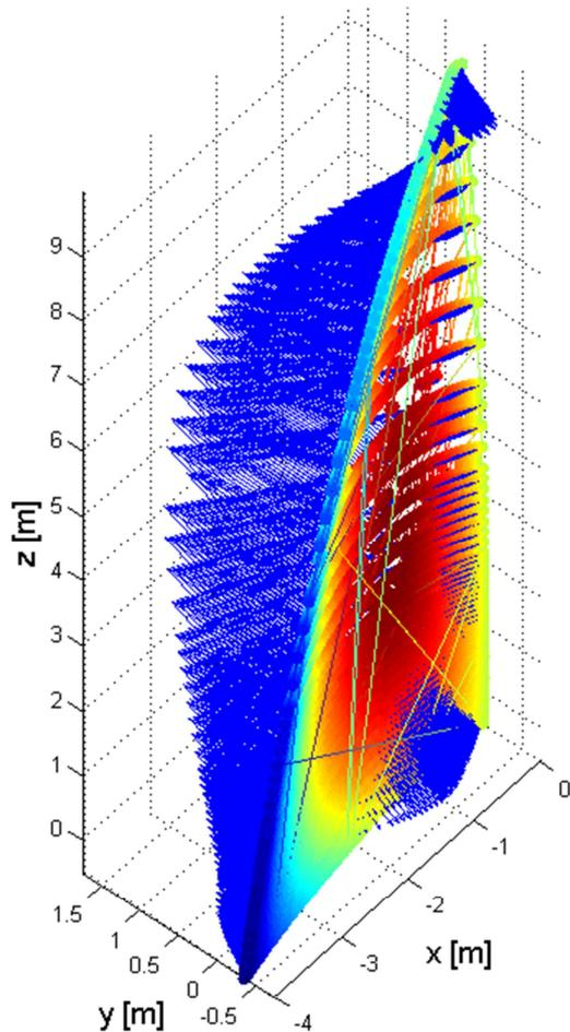
Figure 6 – Displacement vectors of deformed shape of 3D sail. Vectors are magnified for visibility.
