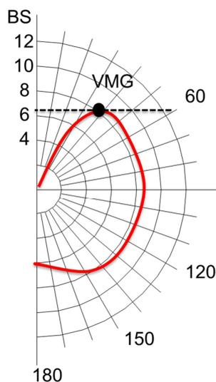
Figure 1. Example of a polar diagram (velocities in m/s and angles in deg).
