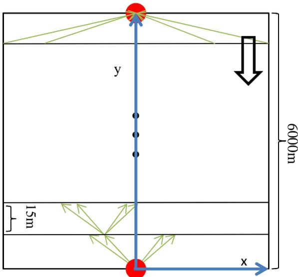
Figure 3. Schematic representation of the course. The y axis is oriented in the upwind direction, and the course is divided into 400 stripes by lines at 15m spacing.
