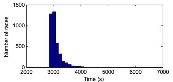
Figure 7. Distribution of time of arrival needed by a boat following the optimum policy.
