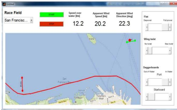
**Figure 3: Screen shot of the touchscreen user interface used for control of the boat and information transfer to the users.**
