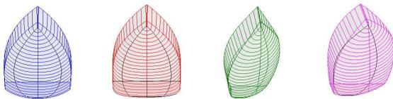
Figure 10: Four random hulls of the Volvo 70 series
