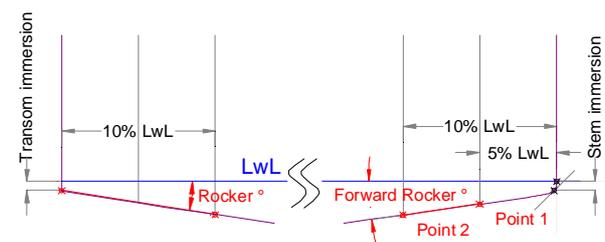
Figure 5: Measurements of the keel line
