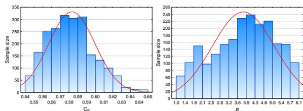
Figure 11: Range of variation of some geometrical measurements (top) and distribution of Cp (bottom left) and Rocker angle (bottom right)
