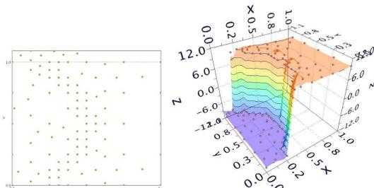
Figure 9: Example of a 3D response surface refined using Lipschitz sampling (Y vs. X graph on the left)
