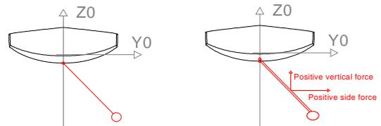
Figure 15: No keel tilt (left), positive keel tilt (right)
