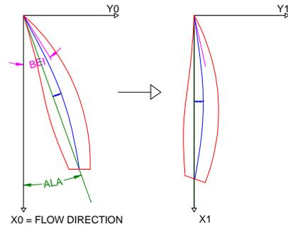
Figure 4: Measurements of asymmetrical wetted shapes
