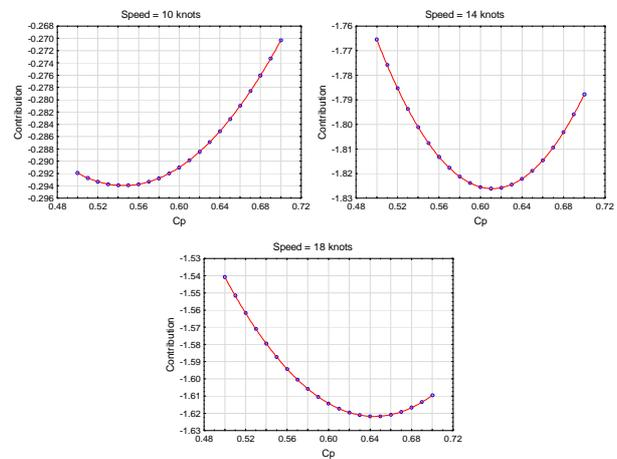
Figure 12: Contribution of Cp to Fpx depending on the Cp value at 10 kts (top left), 14 kts (topright) and 18 kts (bottom)
