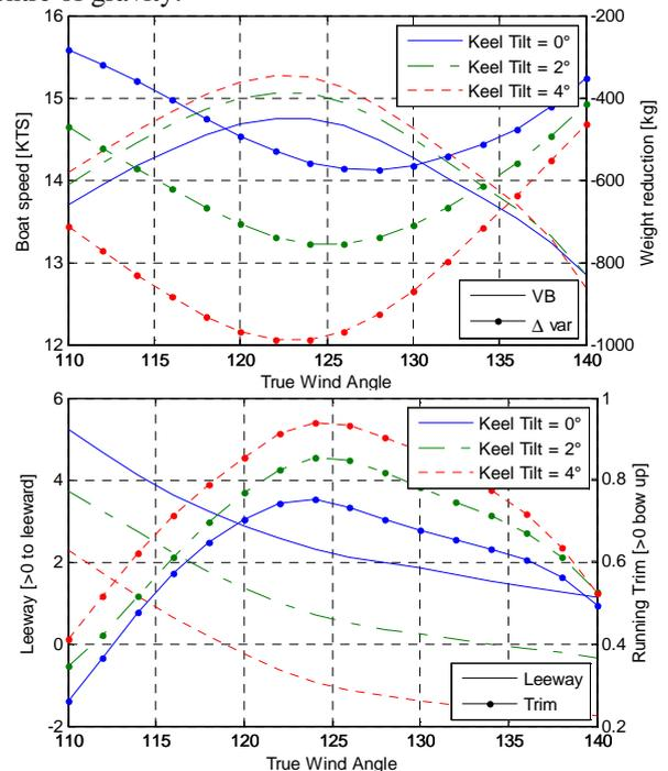
Figure 16: Speed, weight reduction (top), running trim and leeway angles (bottom) for 3 different keel tilts.
