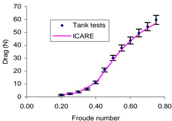
Figure 6 : ICARE solver validation - DSYHS Model 25
