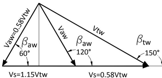
**Figure 1 Wind triangle for downwind sailing**
