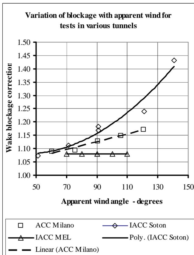
Figure 3 Wake blockage corrections for different tunnels
