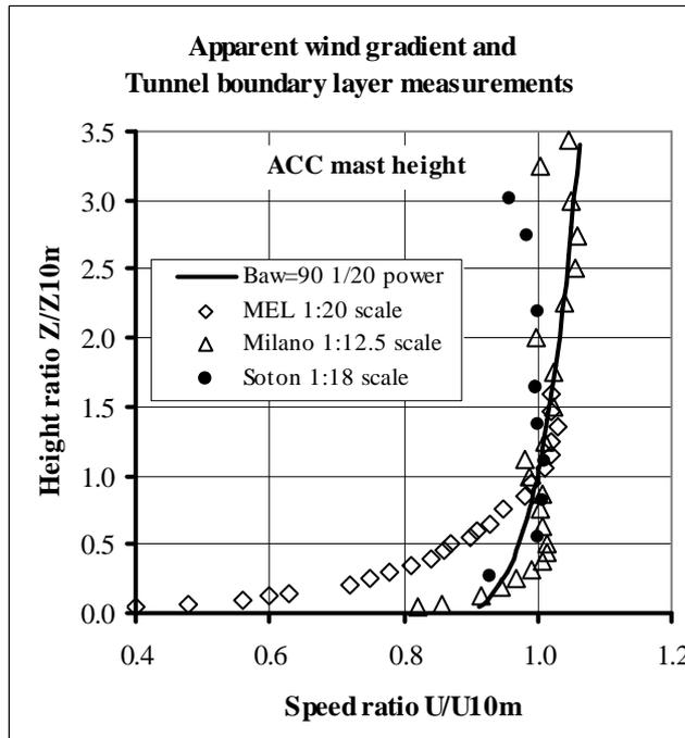
Figure 2 Wind tunnel gradients at the time of the tests
