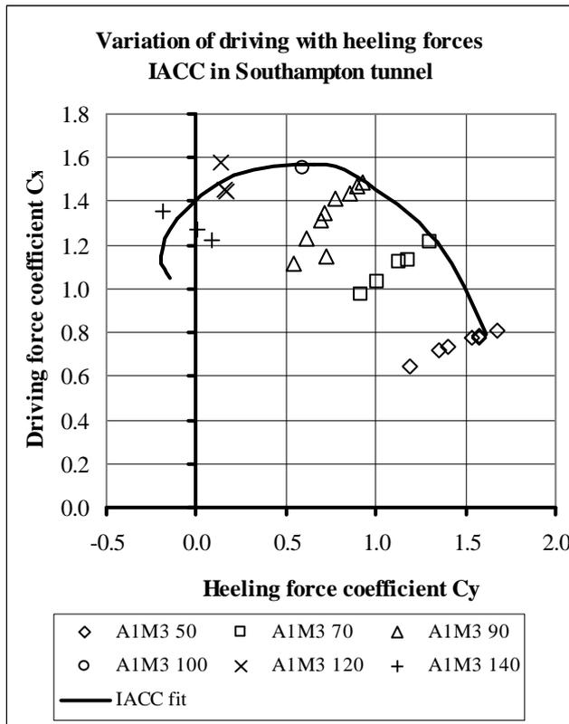
Figure 4 Driving and heeling force coefficients
